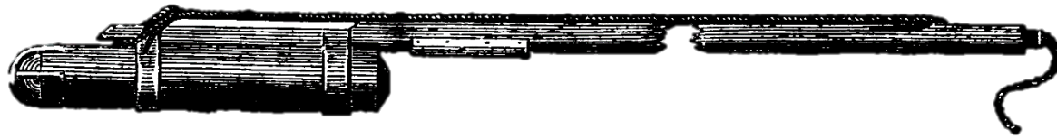
Method of securing a line to Dennett's Rocket
